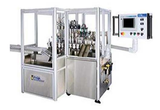
The ProTrac system with speeds to 220 syringes per minute features a race track design, dual filling and closing stations as well as multiple post filling options.
