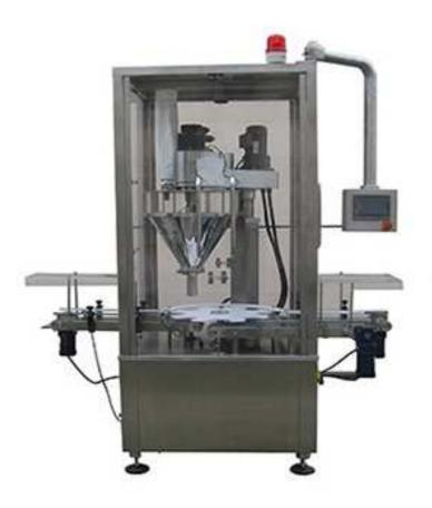
This series could do work of measuring can holding and filling etc it can constitute the whole set can filling work line with other related machines and suitable for filling kohl glitter powder pepper cayenne pepper milk powder rice flour albumen powder soy milk powder coffee powder medicine powder additive essence and spice etc.
