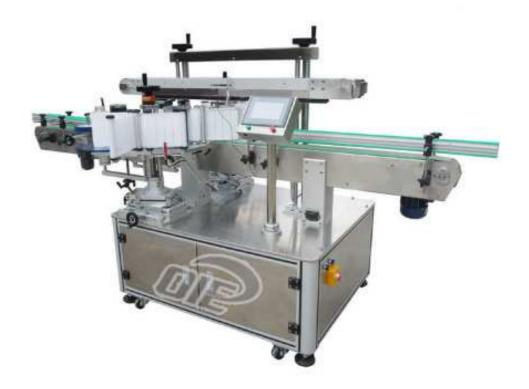
OL-911 is a fully automatic linear labeling machine well designed for round bottles, oval bottles and square bottles single and double sided labeling, such as shampoo oval bottles, lub oil bottles and hand washing bottles.
