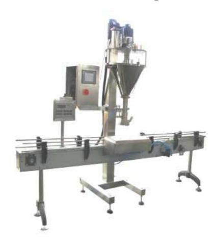
This automatic bottle filling machine is mainly suitable for powder bottle filling with auger filler.
