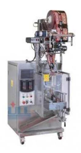
SF-220P Small Powder Packing Machine is suitable for food pharmaceutical, cosmetic, pesticides, plastic products and special products in the industry, automatic, packaging powder materials Such as: food additives, milk powder, soy, flour, protein powder, the powder, mask powder, pearl powder, coffee, powder, cocoa powder, flour, health tea powder, glucose powder, soda powder.
