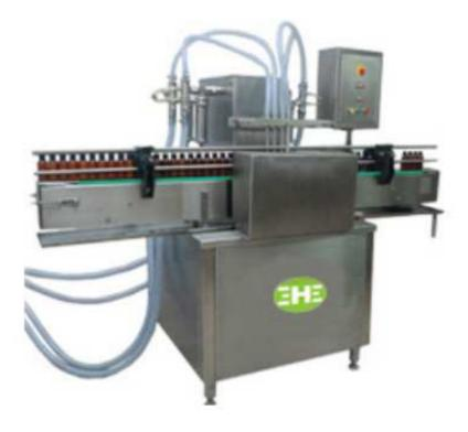
We have wide range of Semi Automatic Four Heads Volumetric Liquid Filling Machine. These kinds of machines are widely used for packaging of Juice, oil, shampoo and syrups used in Pharmaceuticals, Chemicals and Food Products.
