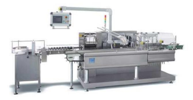
This Automatic Horizontal System Cartoning Machine is suitable for automatic feeding bottle (round, square bottle) into carton (eight for blister or bottle). On line bottle unscramble and feeding, leaflet fold (1-4 folds) and feeding, leaflet detecting, carton opening and forming, products and leaflet pushing into carton, printing batch number, sealing carton with tuck-in or hot melt glue device. Automatically reject lacking of leaflet or product and finished product out.
