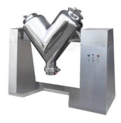
V type dry powder mixer blending machine is suitable for use in the pharmaceuticals, chemical and food industries for mixing powder or granular materials.
