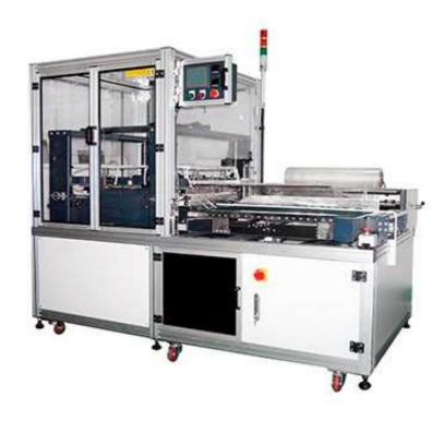
Fully Auto L-sealer, LSA-706A control system adopted PLC & HMI with counting & alerting features, easy maintenance. It has strong sealing line, which is thin & good look.
