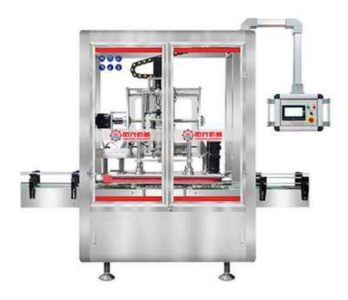
This function is suitable for a variety of geometric shape of the container, with a manipulator, cover speed, no back cover. The machine is suitable for three screw caps and some special bottle caps.
