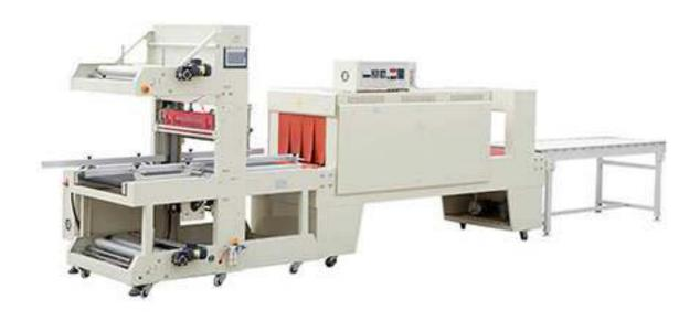
The straight-through sleeve sealing shrink packing machine adopts the direct feeding method, and the packaged articles can be free from the length limit. It is mainly suitable for long things or single shrink packaging of long-length objects or beverages, beer, mineral water, cans, glass bottles and other paper trays and cartons.
