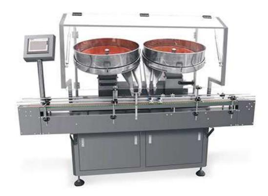
Template Counting Machine sorts and counts grains through several templates, then spins medicines to let them enter filling channel for bottling.
