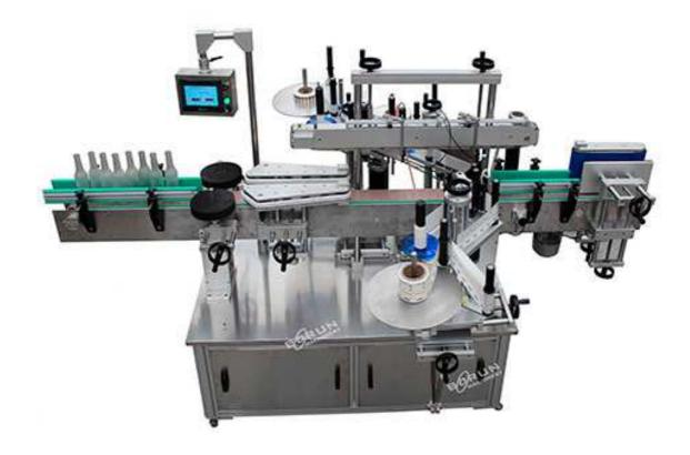
This double sides adhesive labeling machine suitable for the symmetry and non-symmetry containers of wine, foods, cosmetic and label double-faced stickers on the shapes of flat, square, oval, cylinder and other anomalistic containers.
