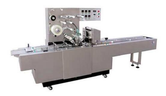
BZT-230B automatic transparent film packaging machine is mainly used for three-dimensional packaging of bulk or multiple pieces of objects such as bulk poker, compressed biscuits, saqima, newspaper post, note paper, and wafer biscuits.
