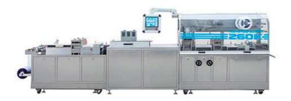
This machine is a new flat-plate fast blister packaging machine designed by our company. It has three independent designs: forming station, feeding station, heat sealing / punching, which distinguishes the structure of traditional tablet machine.
