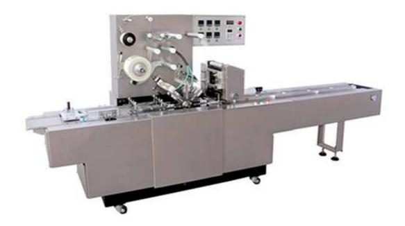
The machine is designed on the basis of absorbing and digesting foreign advanced equipment, using imported digital display transducer and electric components, stable and reliable in operation, a firm steal, smooth an beautiful. It can do automatic packing, feeding, folding, heat-sealing, counting and automatically sticky tear tape. Packing speed can be adjusted steplessly. Changing few parts can wrap different specification (dimension, height, width) of box products.
