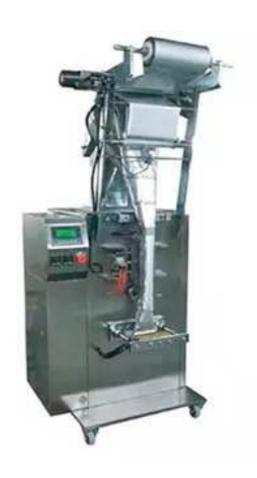
It is suitable for automatic packing of losse nonstick, thick powder products in pharmaceutical, food, chemical industry, such as instant drink, milk powder, MSG, white sugar, instant coffee powder, flour, powder additive, talcum powder, veterinary powder, confiment powder and etc.
