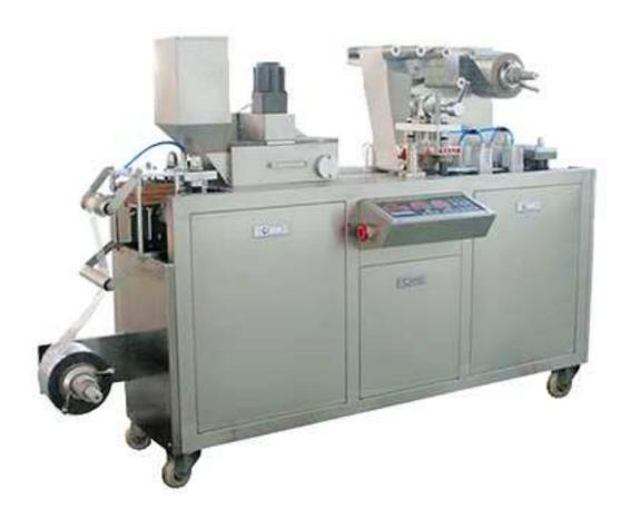
This blister packing machine is special designed for dosage room of hospital, middle or small pharmaceutical and nutrition products factory. It has following features: small machine-body, flat structure mould, easy to operate and change the mould, multifunction, travel can be adjustable, durable in use. It's widely used in pharmaceutical, foodstuff, hardware industry with alu-plastic packing. It's the ideal packing equipment for variety and small batch products packing.
