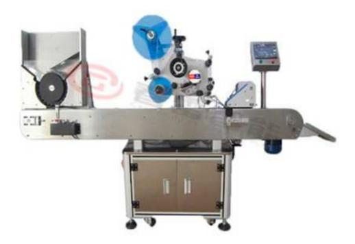
Automatic lipstick labeling machine it is suitable for the labeling of the circumference and half of the circumference of the cylindrical object that is not stable.
