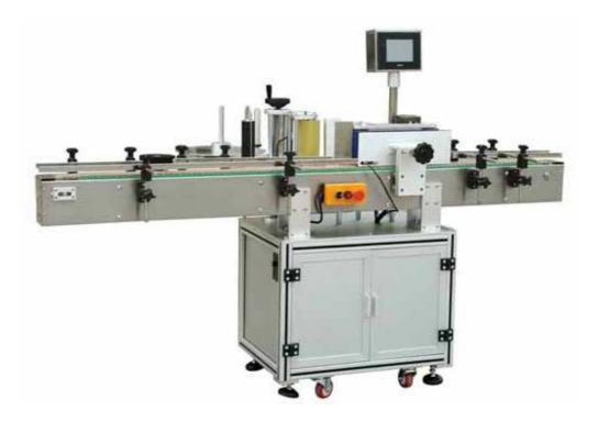
TN-150X intelligent dry adhesive labeling machine adopts programmable control, touch humanmachine interface, step drive sticker. The whole machine is convenient and intuitive, and has rich help functions and fault display functions. Automatic sticker labeling for various round containers.
