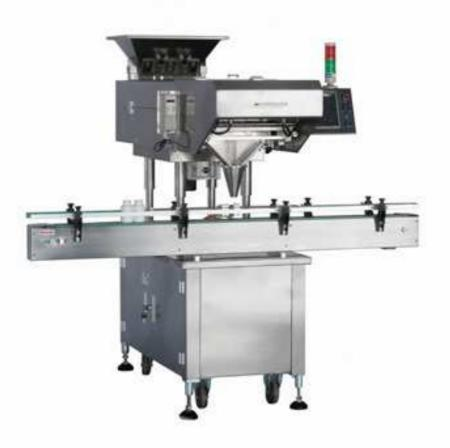
A newly improved Tablet/Capsule counting machine consists of 12 track format with single filling nozzle. Adoption of new Digital Camera System: CCD technology, the CCD-12 combines unerring accuracy with incredible value. The machine handles a wide variety of tablets, caplets and both hard and soft capsules with different shapes and sizes.
