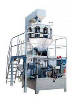
This set of equipment is mainly suitable for automatic counting and packaging of small bags (like medicines, coffee, cereal, cold granules, etc.). After lifting the pouch material into the automatic metering device by the hoist, the computer automatically combines the set quantity, and automatically packs, seals, and outputs the finished product by the bag type packaging machine, and the whole set of equipment is highly automated.
