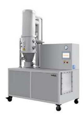
The machine is a multifunctional fluid bed granulator integrating various functions such as top spray, bottom spray and side spray. It has various functions such as mixing, drying, granulating, coating and pelletizing. It is widely used in such industries as pharmaceutical, food, chemical industry, etc.
