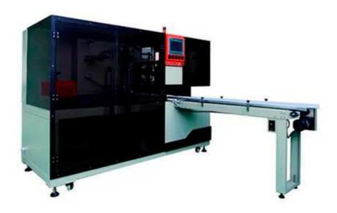
The machine can be combined to use with other production line. This machine is widely applicable to the packaging of various single large box articles, or the collective blister pack of multi-piece box articles (with gold tear tape).
