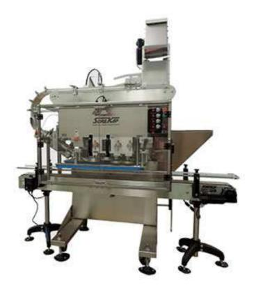
The SK6000X-BF6 is a fully automatic, inline, six spindle capper designed for large cap applications. This machine features NEW Cap Correction Technology to overcome cross-threading issues typical of large caps. Features an innovative belt feed system that eliminates vibratory bowls, overhead hopper loading and time consuming changeovers on a range of flat caps.
