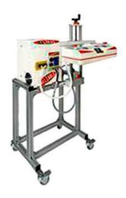
Induction Aluminum Foil Sealing Machine is used for PP, PE, PET, PS, ABS, HDPE, LDPE and glass bottles, which utilizes electromagnetic principle to produce instant high heat to melt aluminum foil that then adheres to the opening of the bottles, reaching the aim of wet-proof, leakage-proof, mildew-proof and extending preservation time.
