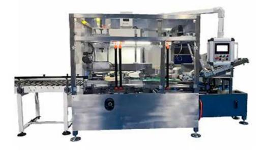
Equipment use: It is a device that spreads the carton and spreads it out, and pushes the product from the side to pack it. This machine can automatically complete the carton unpacking, product stacking and material sorting, automatically push into the box, and then automatically seal the box with high-level automation equipment. The advantage is that it can greatly reduce labor costs and reduce labor intensity.
