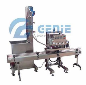
Our spindle type capping machine applies to different materials and standard screw caps, nozzle caps, duckbilled caps, push-in caps. It has torque capping heads, the pressure can adjust.
