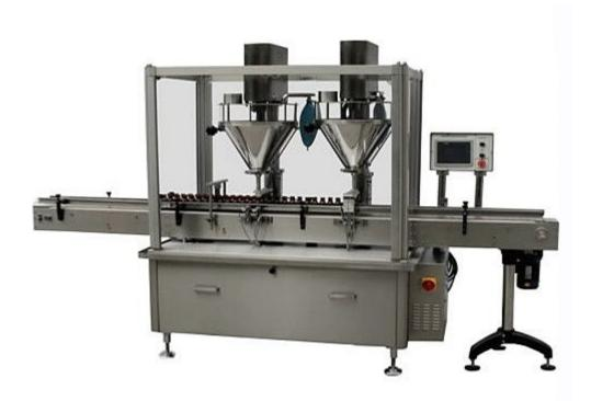
ZH-GZF500 twin head powder filling machine is available for packaging powdery and grainy materials, such as milk powder, monosodium glutamate, solid beverage, icing sugar, and dextrose. What's more, this automatic powder packing machine also fits to coffee, solid medicament, paint, rice flour, etc.
