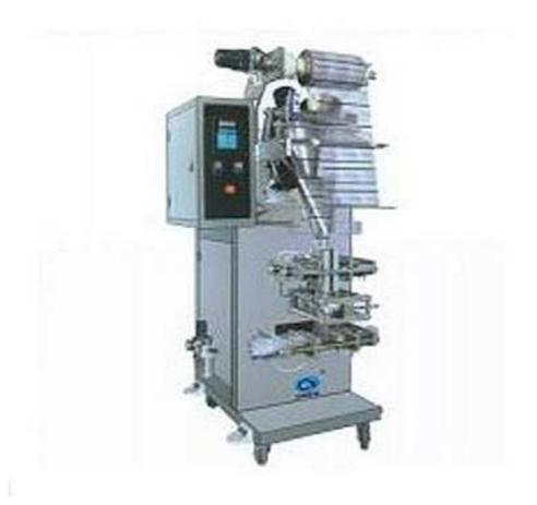
This machine is a trilateral four edge sealing powder packing machine with a set of bag making, measuring, filling, sealing, batch number and cutting bags in one implementation.
