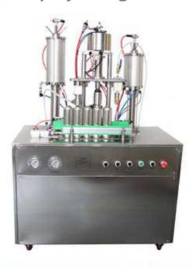
Aerosol Filling Machine is composed of such three parts as: Liquid Filler, Crimper and propellant filling machine (booster pump included). The machine has found widespread application in such fields as pharmacy, healthcare, automobile, environmental protection, fighting and daily chemical, to fill such as mousse, air purifying agent, pesticide, disinfector, fire extinguishing agent, carburetor cleanser and PU foam filler etc. Production capacity: 500-1000 cans/hr
