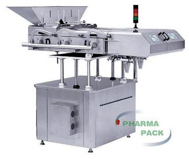
The counter PP-12 is a reliable, high performance machine, designed in conformance with current and proposed GMPs. Having a small footprint, they are effective in maintaining the integrity of a clean room environment. Few change parts are needed for different container sizes (only the nozzle). All product contact parts are made of type 316 stainless steel. And all contact parts can be easily disassembled for cleaning.
