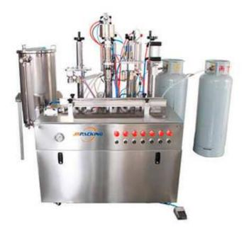
1600C is a automatic aerosol filling equipment, designed with 2 filling machine, 2 gas filling and 1 sealing machine in one working table.
