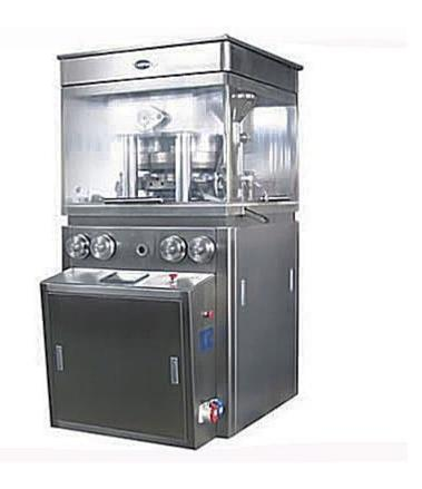
ZP27 double sided rotary tablet press is a kind of punching automatic tablet press. It can press granular raw materials into tablets with different shapes, double colors and letters on both sides. It is mainly used in manufacturing piece prescription in pharmaceutical, chemical, food and electronics industries. When manufacturing double color pieces, it only needs replacing components and adding powder absorbing apparatus, which greatly lowers the cost and increases profit.
