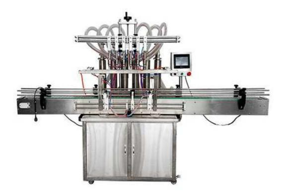
This series of liquid fling machine for daily food, and other types liquid products such as the Water, Wine, Hand sanitizer, Fruit juice, Oil, etc. Piston-type linear fling with high precision filling, easy installation and commissioning, cleaning and maintenance is simple, no dripping and so on.
