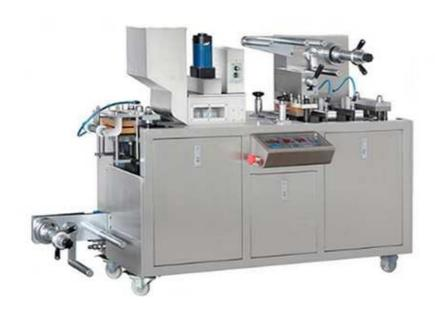
It is suitable for packaging chocolates, butter, biscuits, perfume, essence, face-mask etc with AL/PL, PL/PL materials. It is equipped with a micro-computer control system and frequency converter, with characterized by higher automation and easy operation. career.
