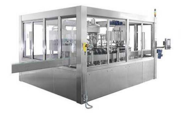
Gallon Filling Machine is highly integrated composed of screw bottle feeding, star wheel conveyance and bottle turning, washing, filling and capping. Featuring novel design, the equipment is clean, safe, stable and efficient at a leading level both at home and abroad.
