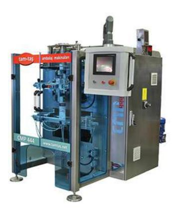
CMP 444 Servo Continuous Motion Packaging Machine is designed to get 130 packs/min for the weight range between 20gr – 1000gr, the size of the pack is 250\*340 mm in maximum, The packs shapes can be Pillow bag, Stand up bag. This machine is designed for the facilities who desire higher speed.
