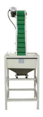
HC-6W bottle cap elevator is special used for transportation cap form low to the higher place of screw capping machine's hopper. It is an auxiliary equipment of cap folding machine, cut machine, plastic drop machine. Can improve productivity.
