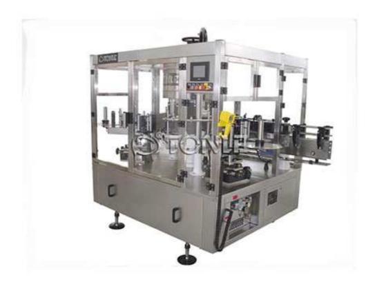
This machine is fully automatic self-adhesive labeling machine. Used for the industries of beer, seasoning, soft drink and so on. It's the necessary labeling machine for the company to upgrade their product and quality
