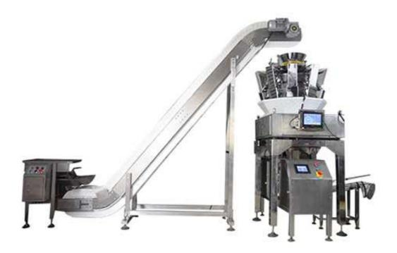
This machine is specially designed for packaging all kinds of granules, such as sugar, salt, seeds, coffee beans, rice, dried fruits, candies, pills, etc., into premade pouches such as flat pouch, gusset pouch, stand up pouch, zipper pouch, doypack, etc.
