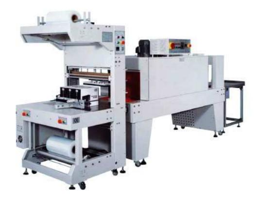
Semi Automatic shrink packing machine is suitable for wrapping of such products as pop-top, mineral water, bottles beer, drinks etc without bottom tray, working with PE film shrink tunnel to pack the goods perfectly
