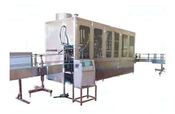
3L-10L water filling machine can be classified into atmospheric pressure filling machine and isobaric pressure filling machine. It depends on the production that customers want to produce. Generally mineral water production line, and pure water production line will choose atmospheric pressure filling machine. Carbonated drink production line, oil production line and fruit juice, fruit tea production line will choose isobaric pressure filling machine.
