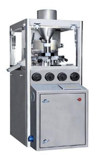
Product description: New high speed single sided tablet press, full automation, compression station is 16, 23, 30 can be selected. Main compression 100KN, pre-compression 14KN, filling accuracy 0.01mm, modular design fully
