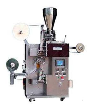
Tea sachet packing machine is a new type of packing machine. The machine is used in many industries. It is widely used for packaging tea, herbal tea, health tea and other small particles in bags.
