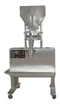
Coffee Filling Machine is suited for various granule in food filling from  $100 \sim 1000$ ml measured by cups volume method. adjustable setting of cups number and no limit filling amount. According with the heath standard material contact parts made in SS304.
