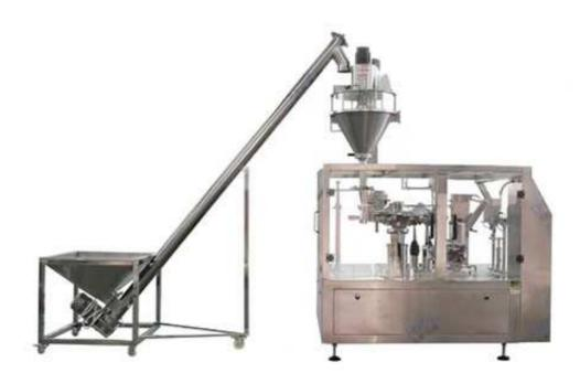
The whole machine is made up of screw feeding machine, silo and eight-station bag feeding unit. All parts adopt SUS304, accord with food safety grade. The working principle is automatic weighing filling, which makes the weighing precision higher and the packing speed faster. The packaging machine can complete feeding, weighing filling, bag feeding, opening, date coding and a series of packaging functions.
