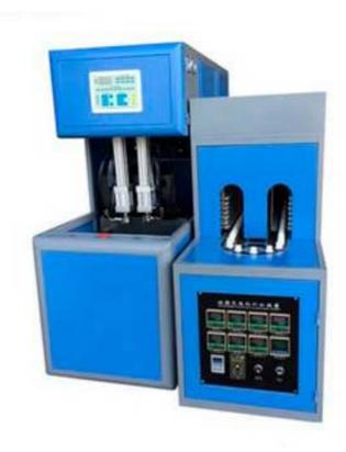
Semi automatic bottle blow molding machine is suitable for producing PET plastic containers and bottles from 0.1L to 20L. It is widely used to produce the mineral water bottle, carbonated drink bottle, Juice bottle, pesticide bottle, oil bottle, daily chemical bottle, cosmetics bottle, wide-mouth Jar, PET can etc.
