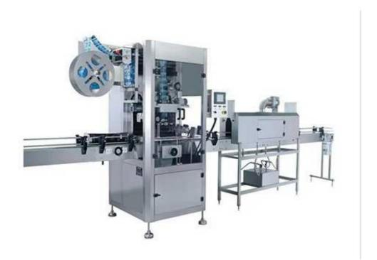
The shrink sleeve labeling machine is most intelligent with operating rapidly and simply for various plastic bottles.
