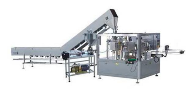
This equipment is mainly composed of bag packaging machine, weighing scale or bowl conveyor, soup filling machine, suitable for fast food industry and food industry. Such as beef food package, beef noodle soup package and other quantitative packaging operations.
